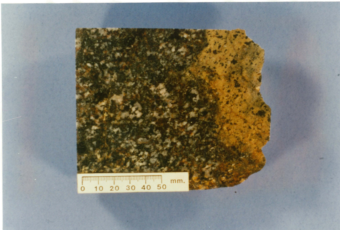
Plate 4-3: Strongly chlorite altered rock flour-rich breccia and nonbrecciated Mine porphyry (Sample WY10, Wildcherry South open pit)
